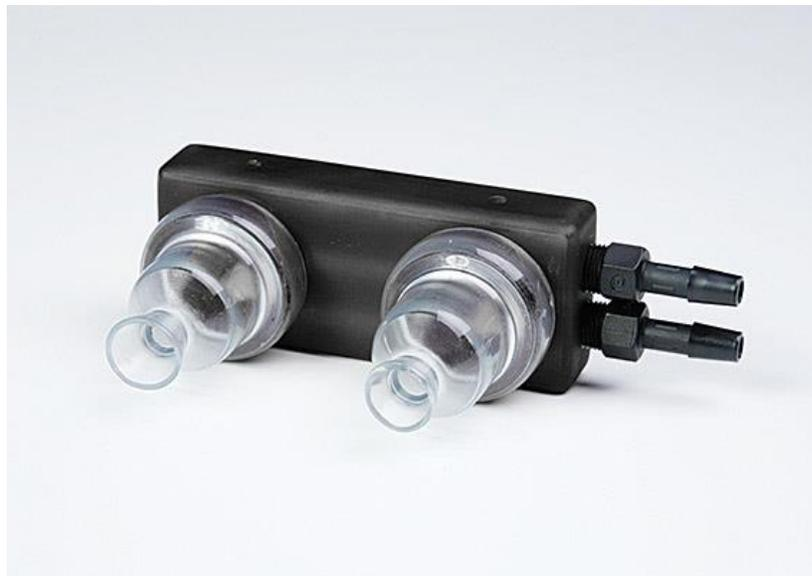
The Biosthesis 300 comes with a dual port breather which can accommodate 2 mice. Other breathers are available under request.
