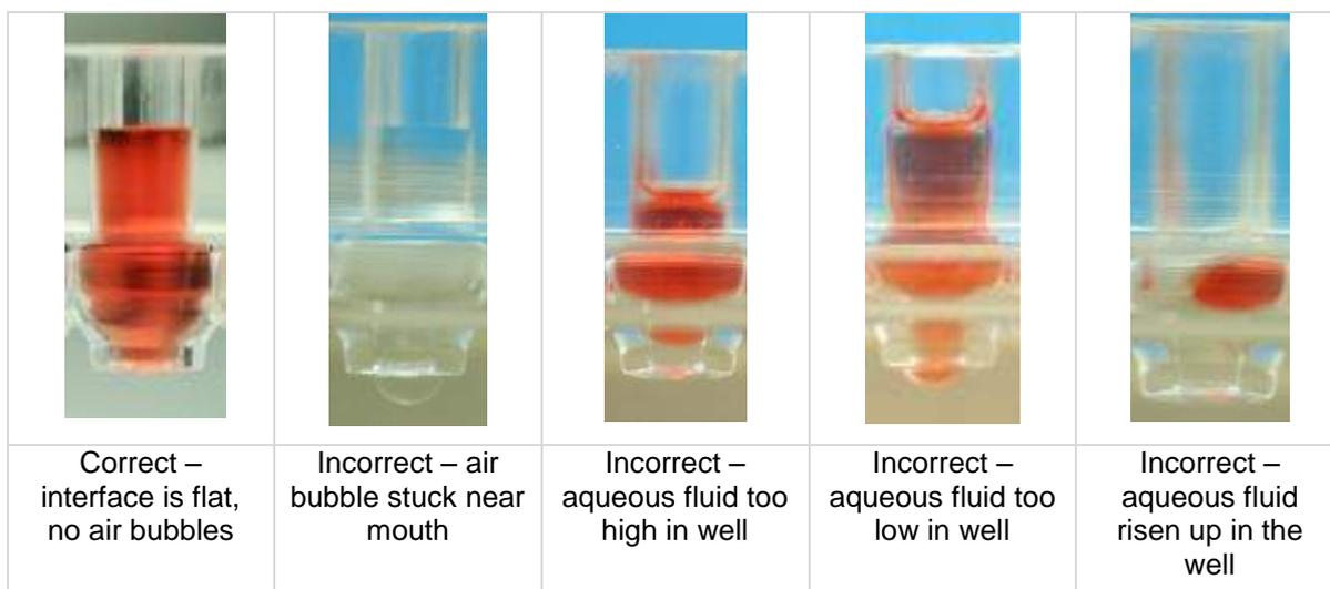
**A:** The aqueous fluid should rest at the mouth of the wells as in the image to the left. To the right, a well is seen with an air bubble lodged, a pendant droplet hanging, or with a receding interface – these are undesirable and require corrective action. Adjustment with a micropipette evens out the hanging drops. There should be no air bubbles visible at the
