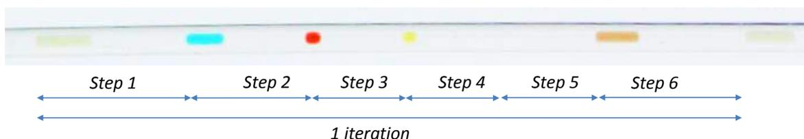
*Bright field image of sequenced droplets in a section of tubing. The above program will produce 50 such iterations. Droplets travel left to right at 5  $\mu\text{L}/\text{min}$  in an FEP tubing of ID 250  $\mu\text{m}$  and OD 800  $\mu\text{m}$ .*
