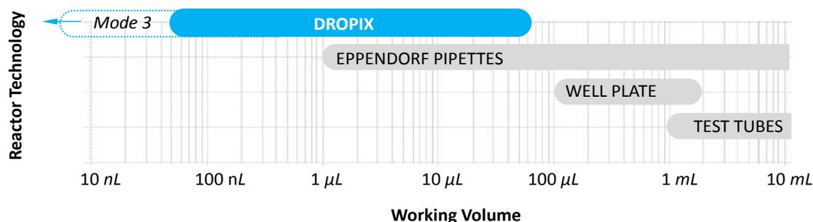
*10<sup>6</sup> reduction in working volume between Mitos Dropix® and various commercially available reactor technologies. A description of Modes follows in the next section.*
