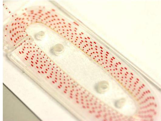
*A Droplet Storage Coil with ~ 450 reactions in a 3 inch<sup>2</sup> area. The fluid flow rate sets the bounds of throughput.*
