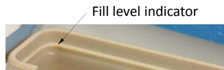
*Fill level indicator in the carrier fluid reservoir. The carrier fluid can be refilled during operation.*
