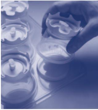
1. Place carrying tray near manifold or vacuum flask and snap off device.
