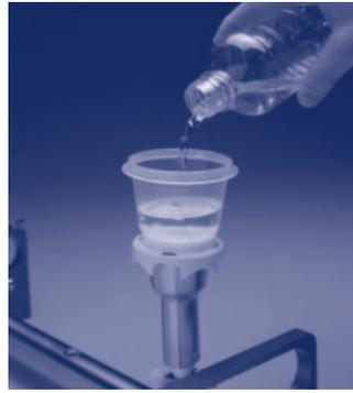
2. Place device onto standard, number 8 stopper, pour sample, and apply vacuum.
