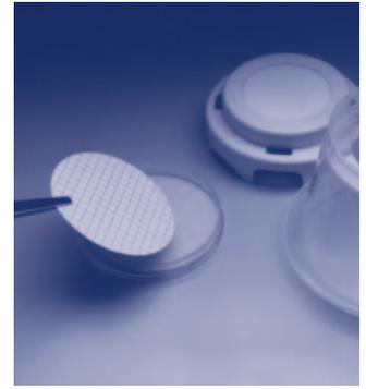
4. Place membrane onto solid or liquid medium and incubate. Discard the base. (It's also recyclable.)
