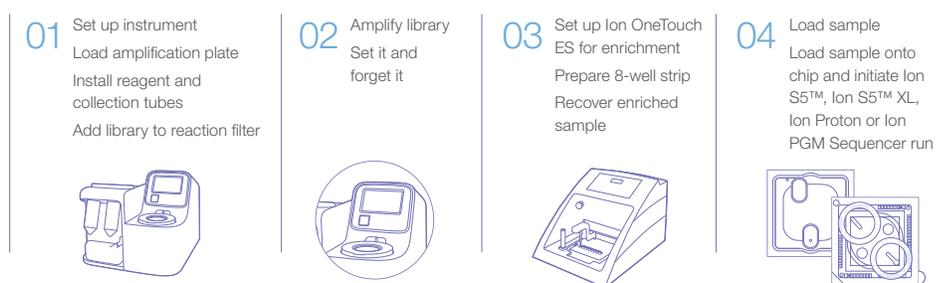
Figure 1. Ion OneTouch 2 System workflow.
