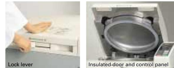
To ensure absolute safety, the door remains locked when pressure or temperature are high. Other safety additions include an insulated swing-up lid, pressure valve, short circuit breaker and scorch-prevention function.
