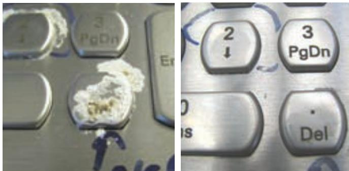
Fig 4. Areas of salt residue and subsequent rust (left photo) are normally easily removed with gentle cleaning with water (right photo).
