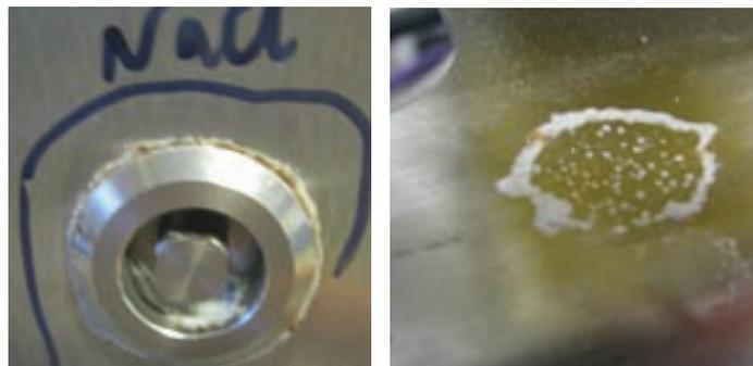
Fig 3. Examples of incipient rust on areas of salt residue on steel surfaces after fogging.
