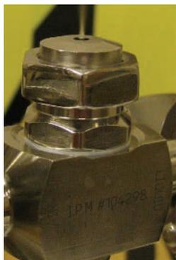
**Fig 2.** A nozzle applying fogging solution.
